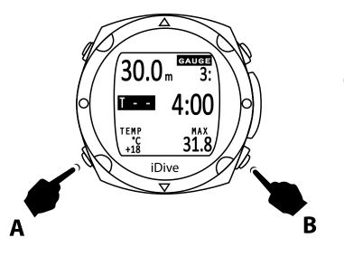
Pressing the **A** button in order to show T + + or T - -. Pressing the **B** button you can decrease the time to a minimum of 0:30
