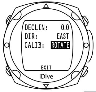
Turn the computer on the horizontal plane up to TILT indication appear.
