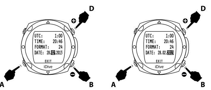
Pressing the **A** button the cursor place of EXIT by pressing the **B** button to confirm the setting returns to the clock function.
