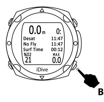
Once on the surface and 10 minutes has elapsed, by pressing the **B** button, you will see some important post-dive data as:
