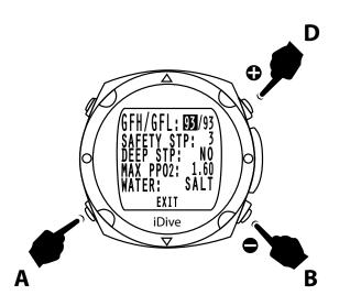
By pressing the **B** or **D** from the main screen menu, you can scroll through the various menu items. When you see the name of a function you must press the **A** key to access the function.
