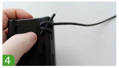
Tighten the bungee carefully and check that the two pins grab the bungee well.
