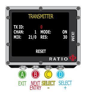
Place the iX3M about 20-30cm from the CC Transmitter (Attention: If you place the CC Transmitter too close to the iX3M the pairing procedure may not work properly).
