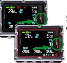
iX3M units that has "iX3M GPS" or "iX3M PRO" label on the top face can be paired with the Ratio® CC Transmitter.
