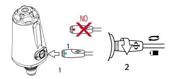
We recommend using a USB wall charger (like a mobile phone/tablet) to recharge the CC Transmitter. However, recharging the CC Transmitter with a PC/Mac is not recommended because there is a risk to only carry out a partial recharge cycle. If using a PC/Mac USB charger (not ecommended), it is essential that the PC/Mac does not interrupt the electricity supply when in stand-by.
