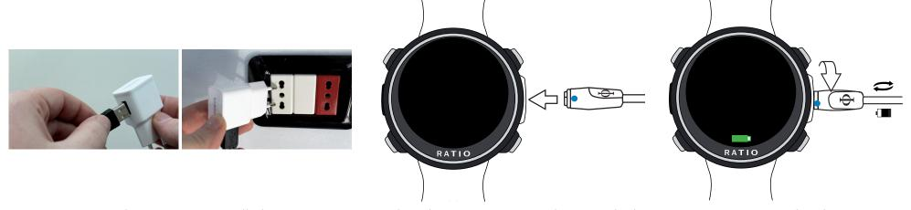
We recommend using a USB wall charger (as opposed to the USB port on a laptop, desktop computer, or similar device) to recharge the iDive. If you do have to use a USB port from a laptop or desktop computer (not recommended), make sure that the device doesn't interrupt the charging cycle by going into standby or sleep mode. Again, recharging the iDive with a laptop or desktop computer is NOT recommended because of the risk of only a partial recharge cycle.
