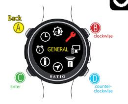
**SETTINGS:** Yes/No. It resets all menu entries to the factory settings. The command SETTING resets all menu and settings (MIX, Alarms, Colors etc.) It doesn't reset the diver's tissues saturation.
