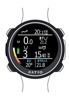
**Warning**: For safety reasons, it is NOT possible to set the FREE mode as main mode if at least 12 hours have passed from the last SCUBA or GAUGE dive. The iDive reset the SCUBA mode automatically if you try to force your dive with the main mode set on FREE.
