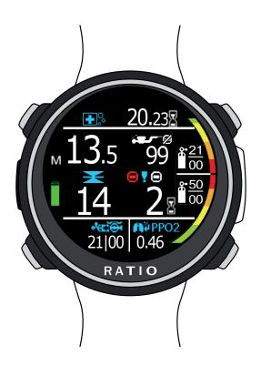
If Deep Stop is enabled: If the function Deep Stop has been activated, this is visualized 5 m before the actual required depth on the screen's central line and will be removed (if not carried out) 5 m after the required depth.
