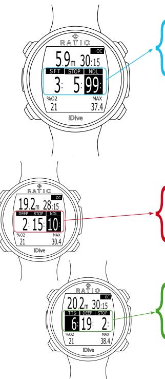
**Safety Stop:** If the Safety Stop (recommended for any kind of dive) is activated, it will be shown on the computer's central line during the ascent starting from a depth of 9 mt.
