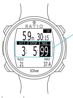
**Safety Stop:** If the Safety Stop (recommended for any kind of dive) is activated, it will be shown on the computer's central line during the ascent starting from a depth of 9 mt.
