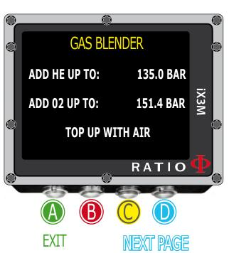
After pressing **EVALUATE** if the mix is possible with the inserted settings, the iX3M will show the procedure to follow to obtain the desired mix.
