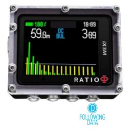
The yellow lines represent the nitrogen levels . The green lines represent the helium levels (if present) The blue line represents the environment pressure in the surface at the dive's beginning.
