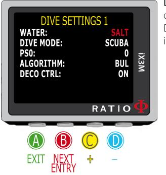
**DECO CTRL:** (ON/OFF): If activated (ON) the iX3M will not allow you to carry out a new dive during the 12 hrs after a dive in which there have been several deco violations. The DECO CTRL deactivation (OFF) is not recommended and will remain permanently in the iX3M Logbook.
