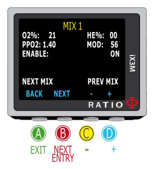
**O2%:** It Indicates the Oxygen % contained inside the mix. **HE%:** It Indicates the Helium % contained inside the mix.
