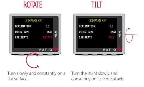
For a correct survey, carry out the calibration far from magnetic field sources i (PC, TV, light poles etc.)
