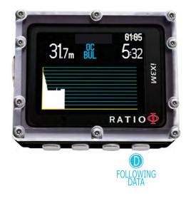
Current depth: (left) with coloured alarm code when passing the gas MOD, the mandatory stop and the depth alarm. Dive Mode: (centre) Kind of dive and used algorithm: OC= Open Circuit, CCR=Rebreather BUL= Bühlmann ZHL-16 B, VPM= VPM-B Dive Time: (right) Runtime in minutes:seconds
