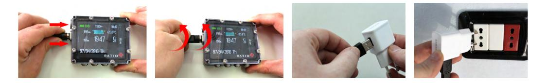
To recharge the RATIO iX3M we recommend to use a USB wall charger (like the one of your mobile/tablet). If you decide to use a PC USB plug (deprecated), make sure that the PC doesn't interrupt the electricity flow once in stand-by.
