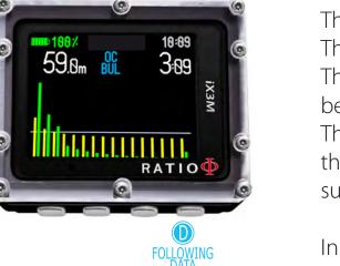
The yellow lines represent the nitrogen levels . The green lines represent the helium levels (if present) The blue line represents the environment pressure in the surface at the dive's beginning.
